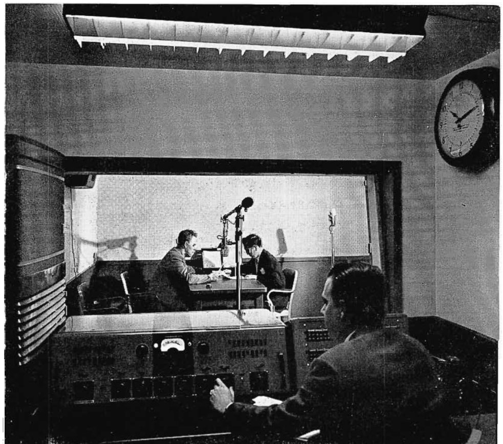
FIG. 5 (below). Most of the KSD newscasts, chain-break commercials and interviews go out from Studio "C", which is shown here as it appears from the control room. RCA 76-type Consolettes and LC-1A Monitoring Speakers are used in all control rooms.
