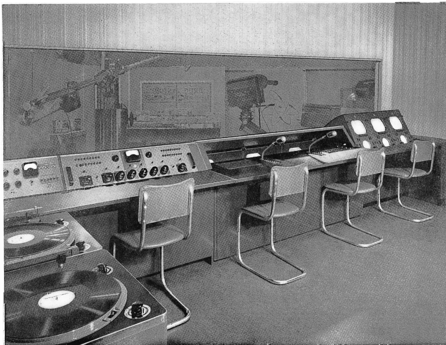
FIG. 5 (below). This station also employs the audio system setup shown in Fig. 4, with a different arrangement of equipment. Note, 70-D Turntables, located at the left, audio TV control at center, program director's console and camera control units at right, form a single operating unit.
