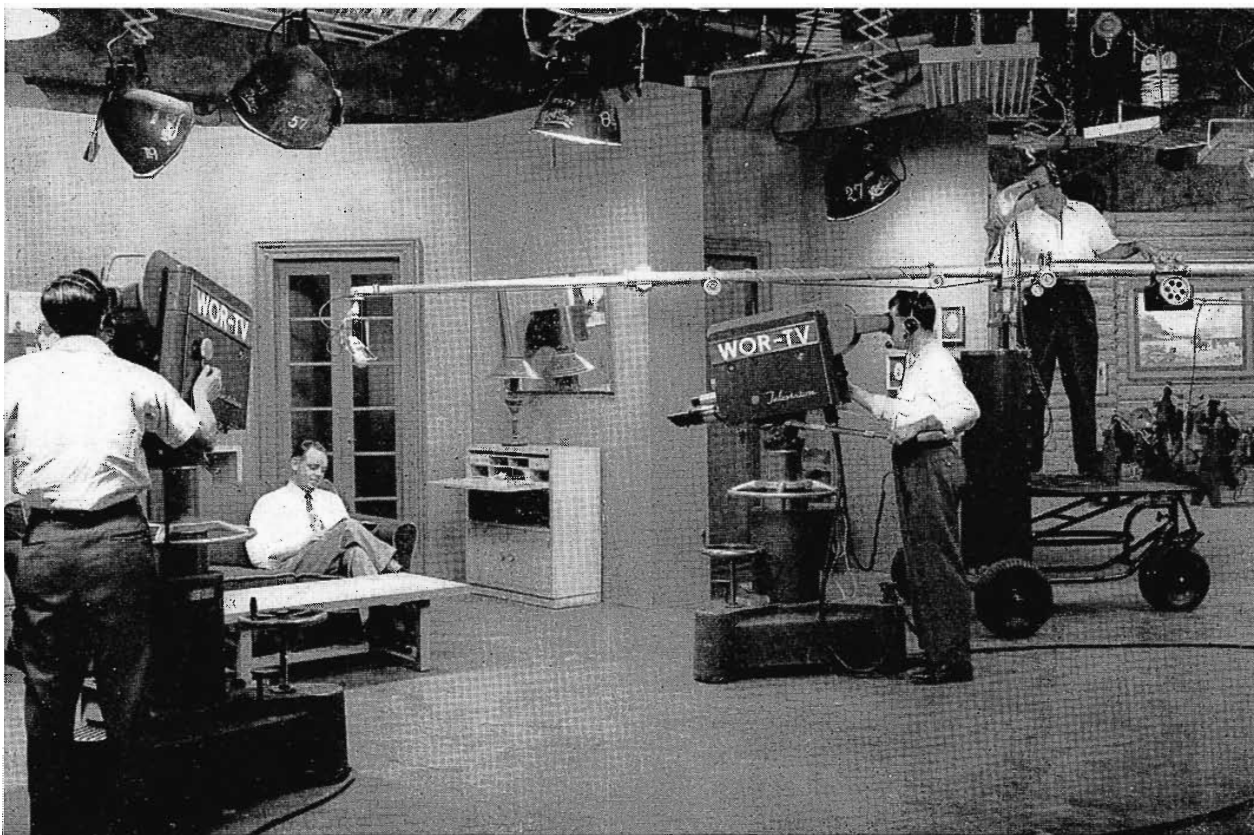
FIG. 7. A flexible and easily-operated boom stand is an invaluable piece of TV studio microphone pick-up equipment. In this photo (courtesy of WOR-TV) boom operators may be seen extending the microphone to a desirable pickup position.
