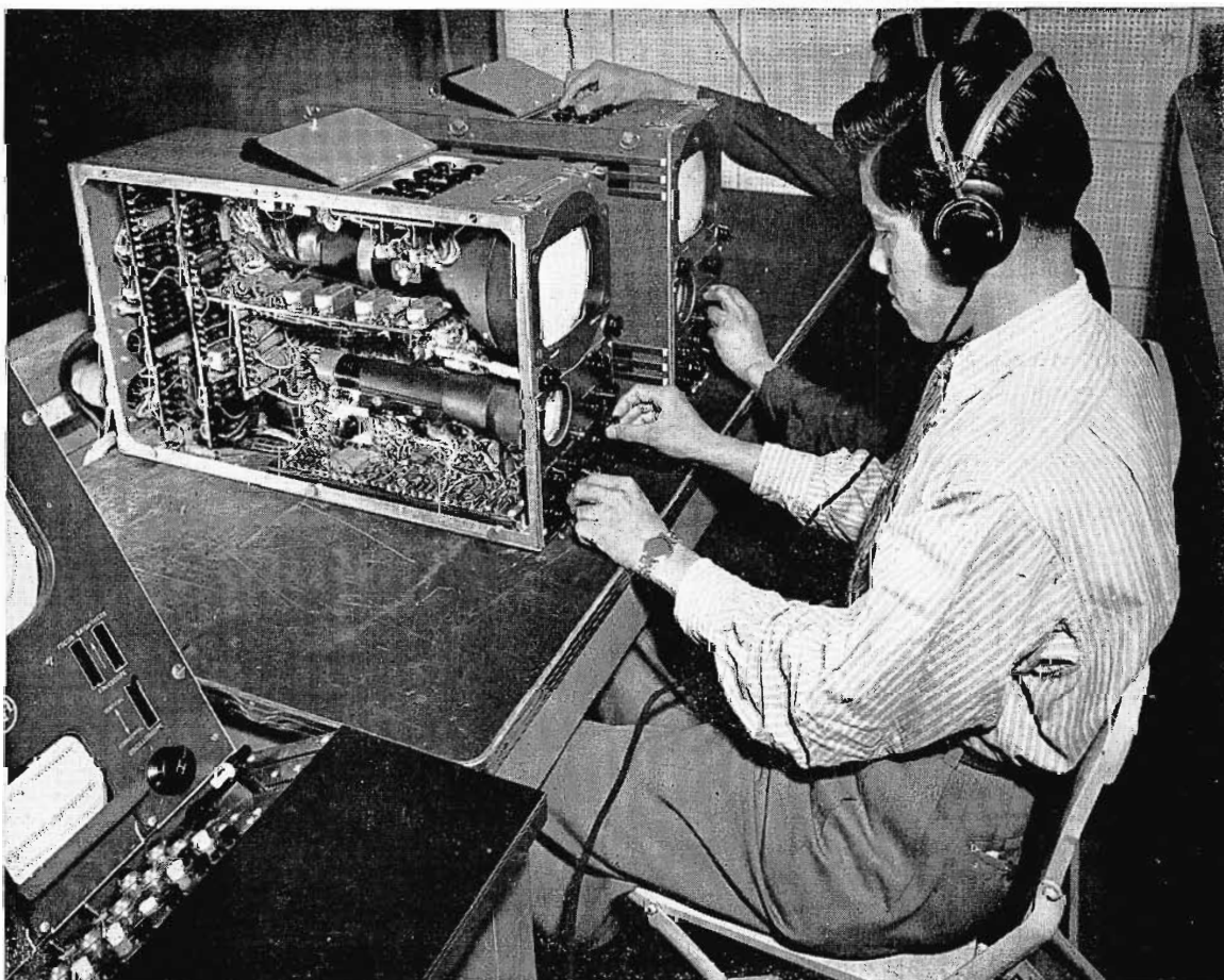
FIG. 7. View of video operators adjusting XHTV's Camera Control Units. Visible at extreme left is part of the TS-10A Studio Camera equipment.
