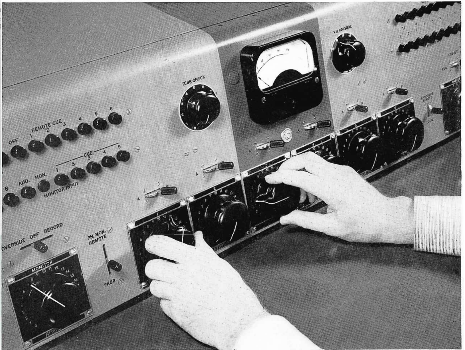
FIG. 2 (above). The RCA 76-B5 Consolelette serves as an important part of the TV audio system. It incorporates four pre-amplifiers feeding a six-position mixer system.
